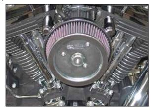
11. Install the K&N® air filter onto the base plate and secure with the provided hardware. NOTE: Be sure to apply one drop of thread
