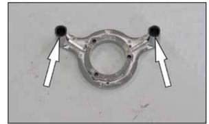
7. Install two of the provided o-rings into the K&N $^{\circ}$  crankcase breather plate as shown.
